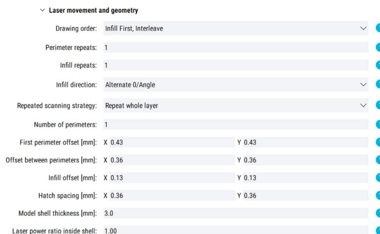
Fig. 2.18 Laser movement and geometry section.
