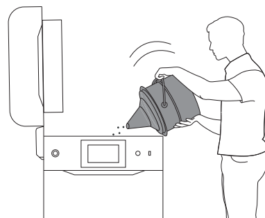
Fig. 2.5 Filling the print chamber with powder using a funnel.
