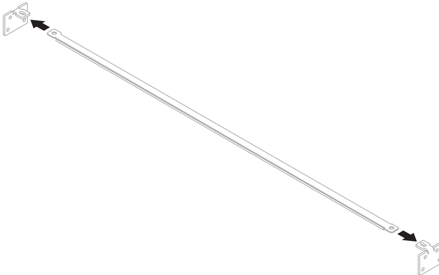
Fig. 3 Positioning the Recoater strip.
