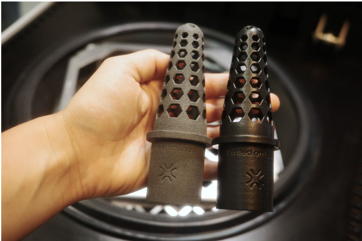
Grey Sinterit parts printed on Lisa X & finished with the DyeMansion VX1
